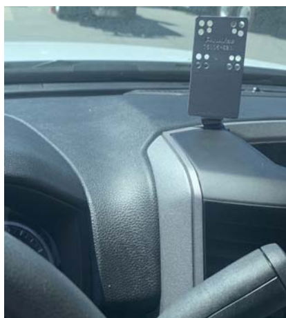
InDash Mount Installed
